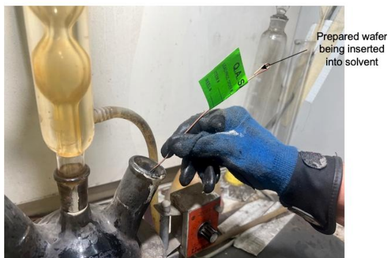
Figure 20 – Wafer boil test setup
