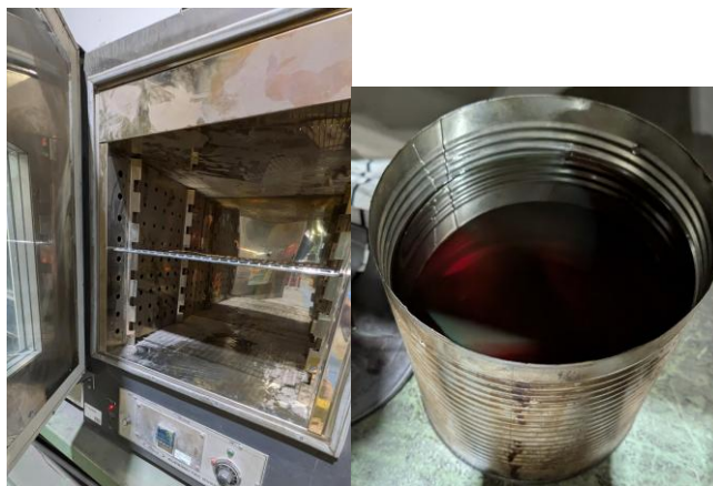
Figure 49 – Oven (left) and oil (right) for oil immersion test
