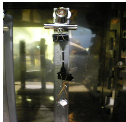
Figure 22 – “Dog-bone” specimen in oven attached to supporting apparatus with weight
