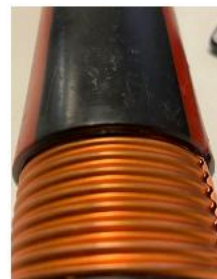
Figure 27 – Measuring and calculating corrugation lay factor
